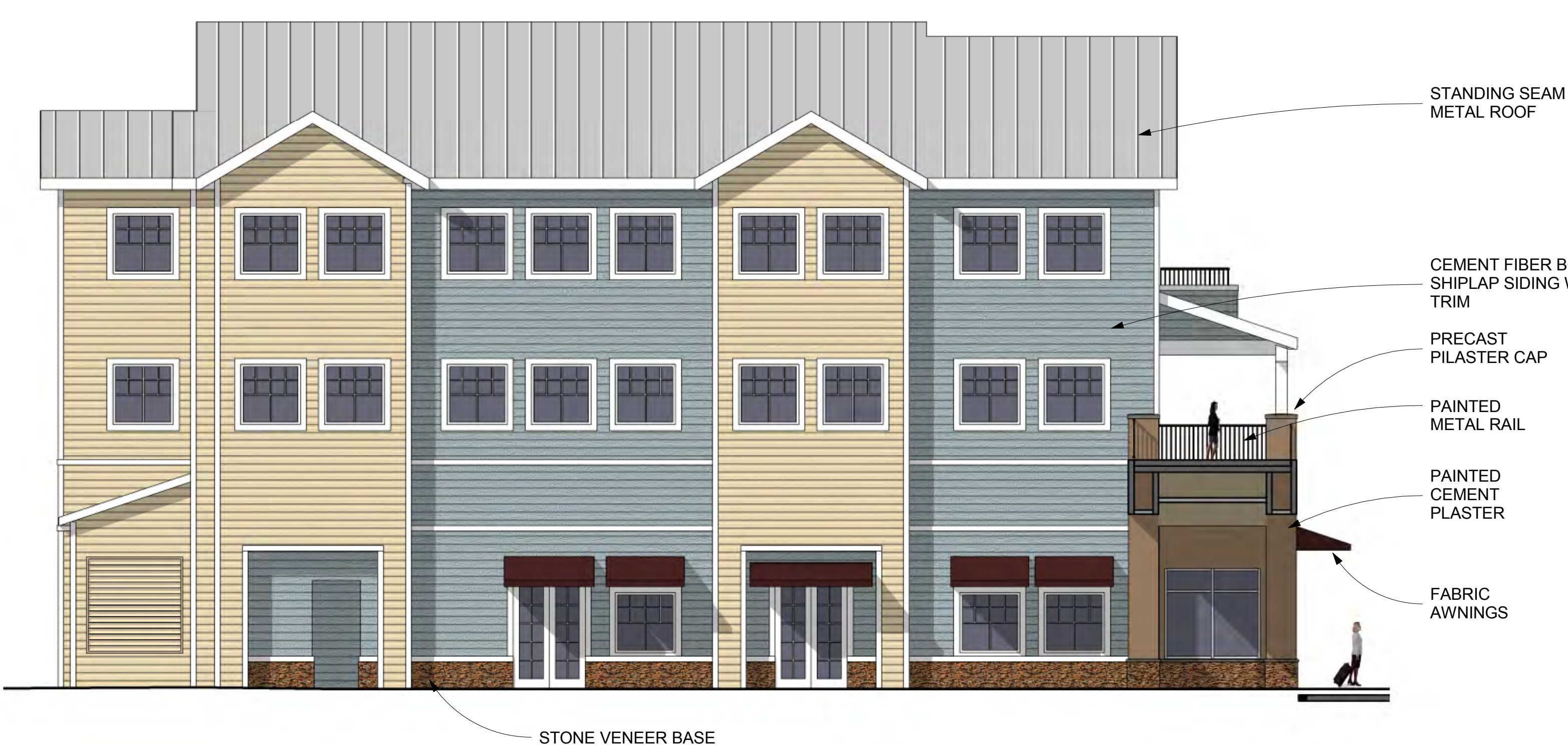
BUILDING 6 WEST ELEVATION 1/8" = 1'-0" 6
