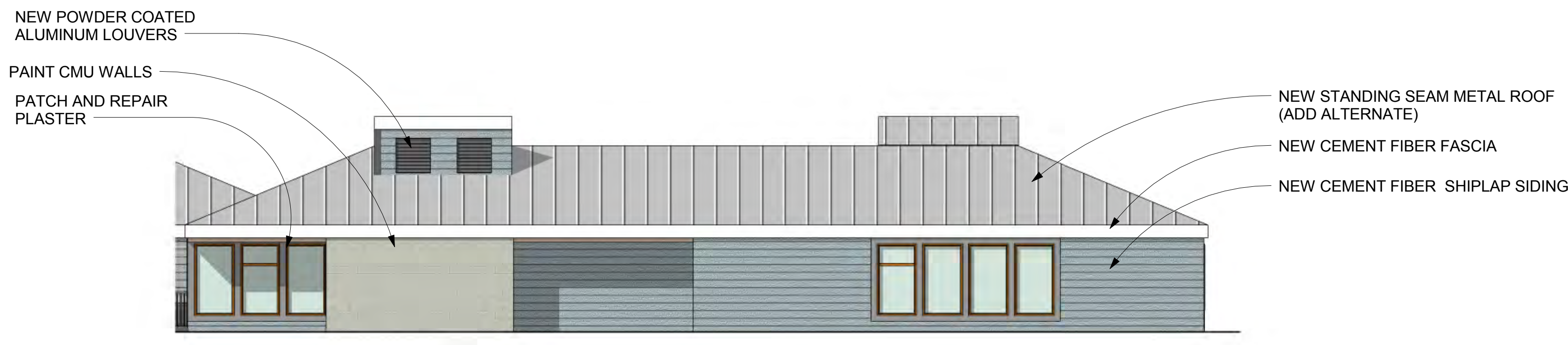
BUILDING 3 - WEST ELEVATION 1/8" = 1'-0" 8
