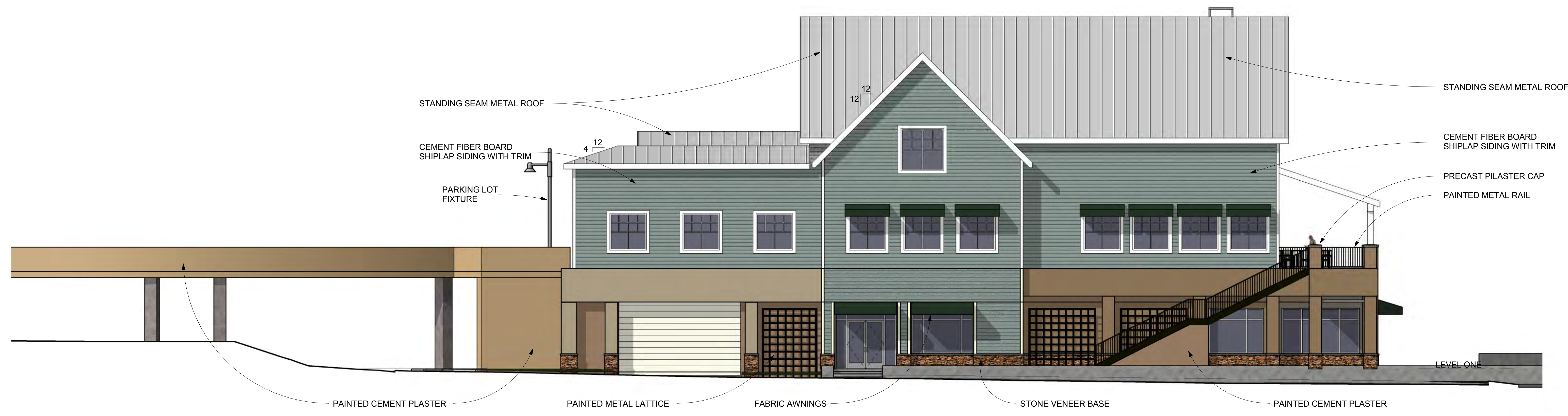
BUILDING 9 WEST ELEVATION 1/8" = 1'-0" 3
