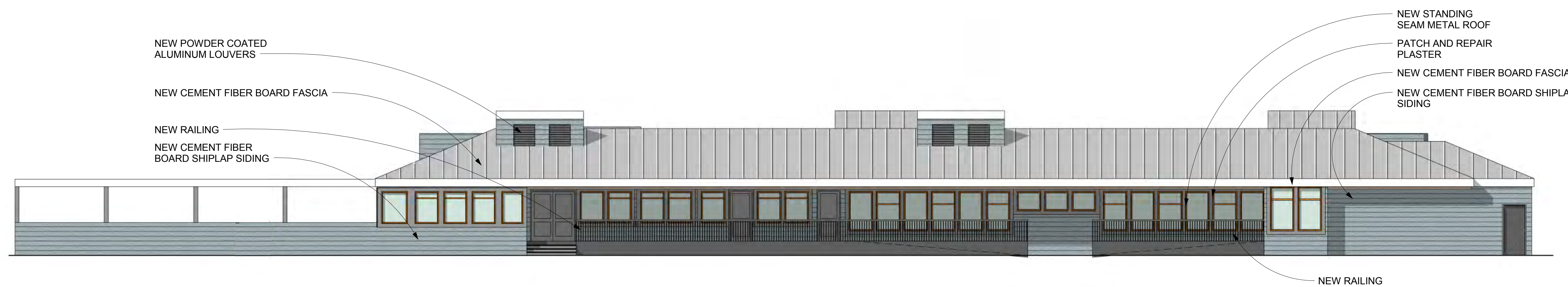
BUILDING 2 - EAST ELEVATION 1/8" = 1'-0" 1
