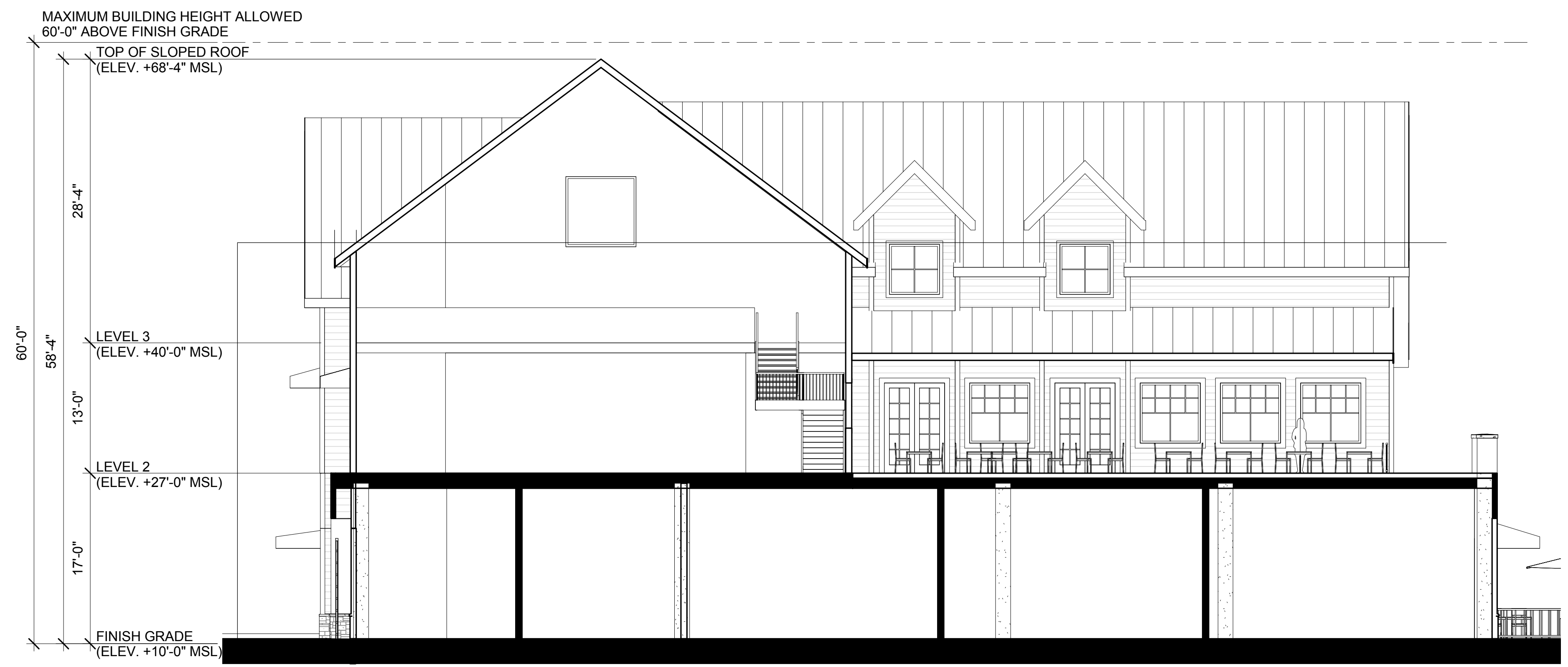
BUILDING 9 EXISTING GRADE: 8'-6" TO 11'-0" ABOVE MEAN SEA LEVEL NEW PAD ELEVATION: 9'-6" ABOVE MEAN SEA LEVEL NEW FINISH FLOOR ELEVATION: 10'-6" ABOVE MEAN SEA LEVEL PROPOSED MAXIMUM BUILDING HEIGHT: 58'-4"
