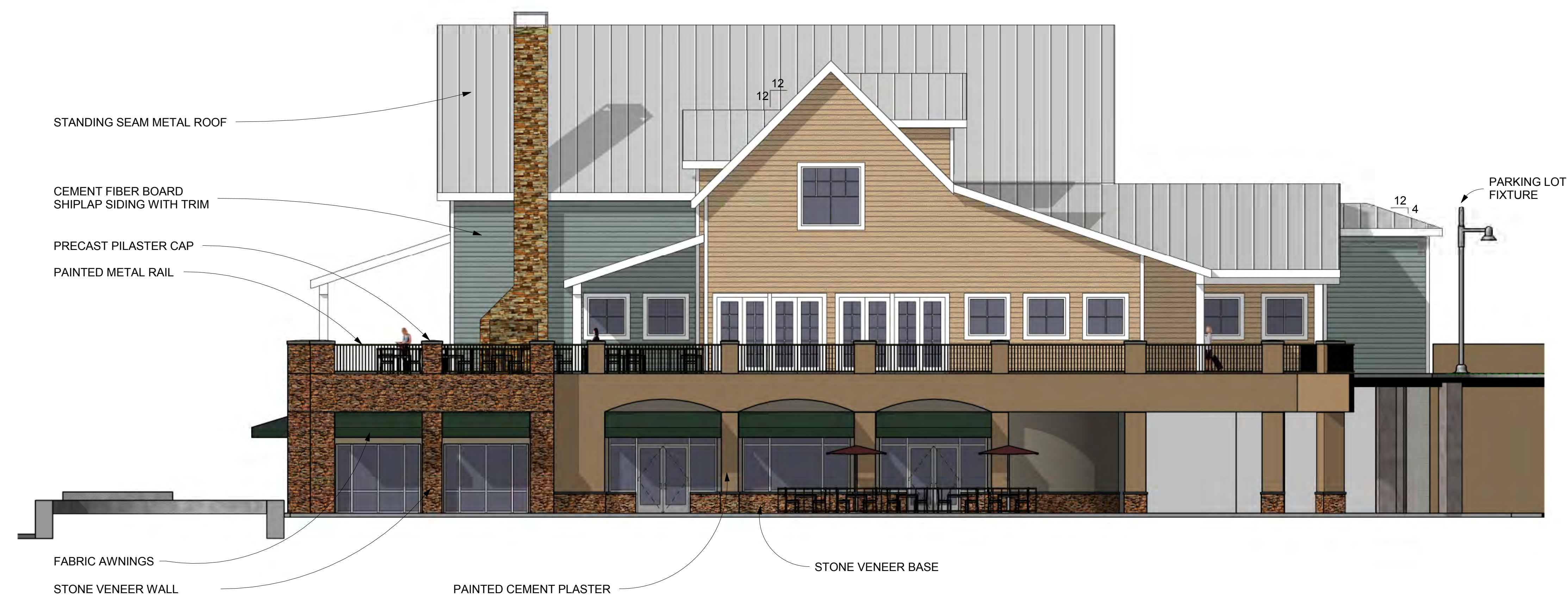
BUILDING 9 EAST ELEVATION 1/8" = 1'-0" 3
