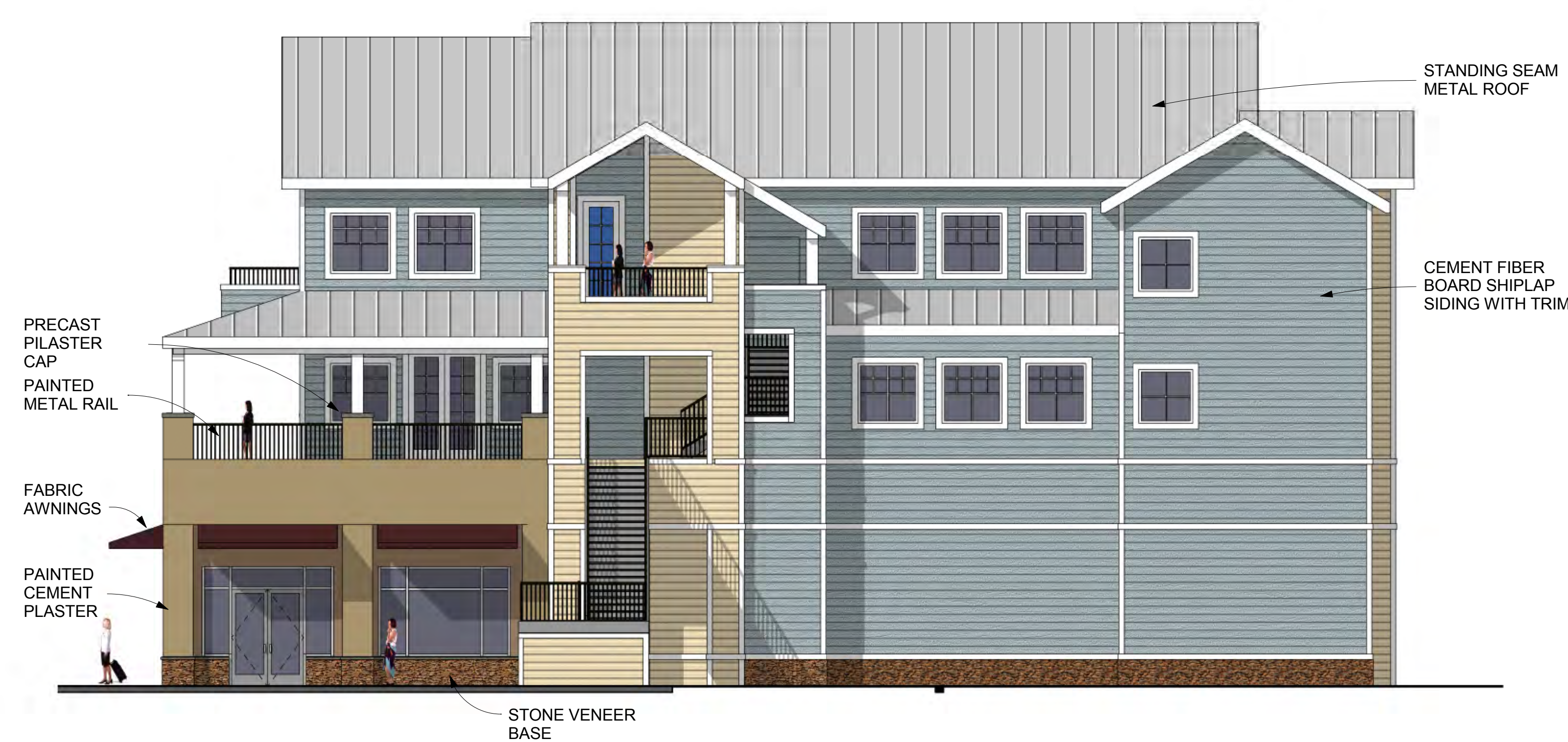
BUILDING 6 EAST ELEVATION 1/8" = 1'-0" 4
