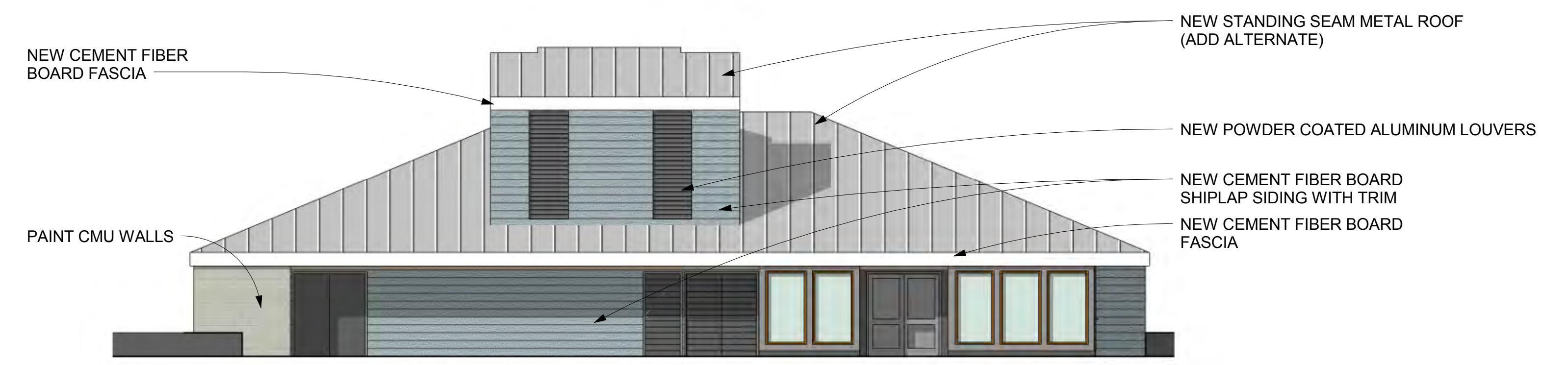
BUILDING 4 - NORTH ELEVATION 1/8" = 1'-0" 6
